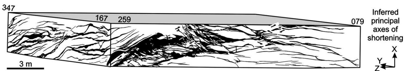
Fig. 8. Block model of a vein array in the footwall of the Thompson fault-fill vein (1045 RL). The east-striking section displays less than 45° dipping en echelon arrays of sigmoidal veins within brittle-ductile reverse fault zones. Veins in the centre of the east-striking section are rotated about 45° west-dipping reverse fault zones. Vein geometries vary along strike and dip and veins interlink to form a mesh. Kinematics of structures suggests sub-horizontal east-west shortening and vertical extension.
